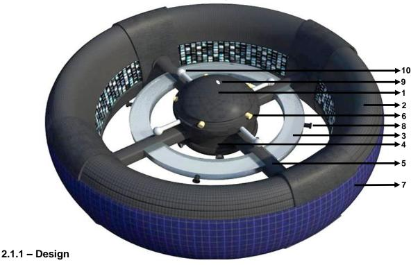
Its design consists of the following key structural components: the central sphere, the residential ovular torus, the agricultural/storage disks, the elevator cylinder bay, and the transportation and structural support spokes.
