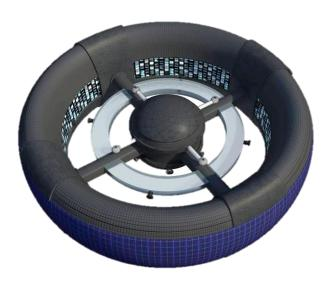
Phase 7: The 1g residential torus is complete. The construction of the micro-g spheres' framework, protruding from the central sphere, will now be carried out. Thrusters for station keeping will now be placed on the rotating band on the sphere. The disks and torus will now commence initial rotation at 1.0 RPM. Artificial Gravity will now be applied. Interior construction of the residential torus will now begin.
