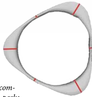
Figure 2.1.7 Each section of the torus contains all gravity levels so they can maintain normal operation even in an emergency.
