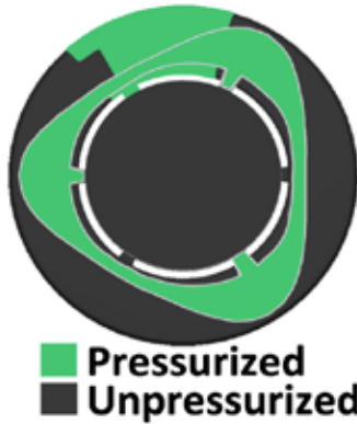
Figure 2.1.8 The majority of the manufacturing core is unpressurized to minimize material costs.
